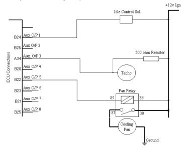
**NOTE:** All outputs actually connect to ground. This means that any device being controlled must be connected to power at the positive end and to the ECU output at the negative end. Each output can sink up to 1 amp.
