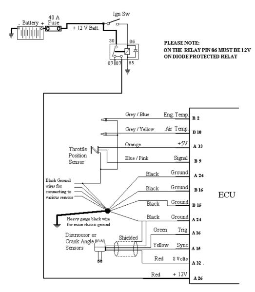
Please Note that there are 2 red wires. The thicker of the 2 wires is connected to the ignition 12 volts and the thinner one is an 3 volt supply which goes into the shielded section of the loom and is used to power the trigger sensors. All black ground wires are joined inside the loom.
