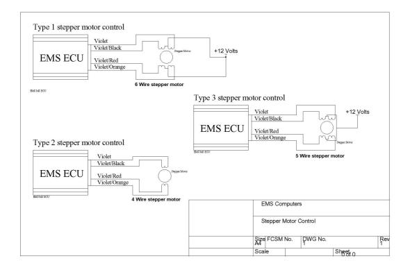
**Note:** If you are not using the stepper motor output wires then you must ensure that they are insulated to prevent short-circuiting. Shot-circuiting these wires will damage the ECU.
